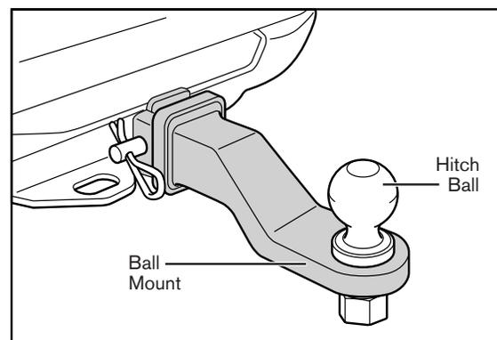
Most hitch balls have the size stamped on the top of the ball. The required hitch ball size is stamped on most trailer
