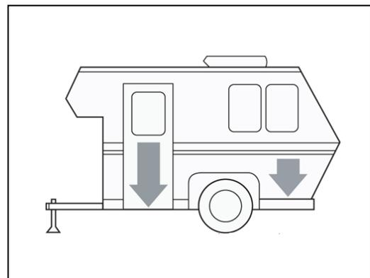
**WARNING** -The trailer load should be balanced equally from side-to-side. Unequal side-to-side loading can negatively affect handling and braking. Once in place, all cargo should be firmly secured to prevent shifting. If the load should shift abruptly during braking or cornering, it could quickly affect the handling of your vehicle and cause a very unsafe situation.
